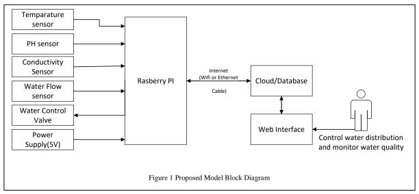
5 sensors where three of them are for water quality monitoring and two of them are for smart water distribution. The sensors are controlled by the raspberry Pi controller which is connected to the internet via Ethernet cable or Wi-Fi. Using the internet, Raspberry PI sends and receives the data or command to/from Cloud or Hosted Database for performing the real-time operation. A user can control system using web interface.
